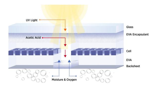
Although moisture and water wear away at the entire outer surface of backsheets, they crack more quickly in the area between solar cells where sunlight shines through. NIST researchers propose that degradation is worse there because acetic acid, which forms when sunlight hits the the rubbery upper layers, can pass between the solar cells towards the backsheets, causing them to decay from the inside out. Credit: N. Hanacek/NIST
