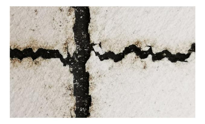
Cracks often form on solar panel backsheets in straight lines, along the gaps between solar cells. Credit: NIST
