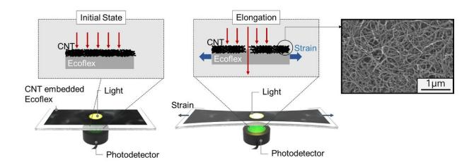
Figure 2. Schematic diagram of the sensor based on the optical transmittance changes of the CNT-embedded Ecoflex thin film. Credit: The Korea Advanced Institute of Science and Technology (KAIST)
