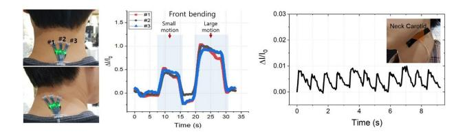
Figure 4. Posture monitoring using 3-axes strain sensor array, and pulse monitoring on the carotid artery. Credit: The Korea Advanced Institute of Science and Technology (KAIST)
