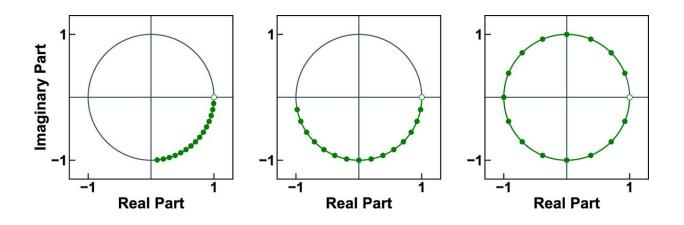
Here are three examples of 16-point chirp contours on the unit circle. The ICZT algorithm developed by Iowa State engineers can work with all three while the one previously used can work only with the last contour. Credit: Alexander Stoytchev.
