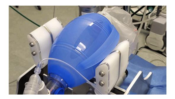
The latest version of the MIT E-Vent team's emergency ventilator design undergoes testing in their lab. Credit: MIT E-Vent Team
