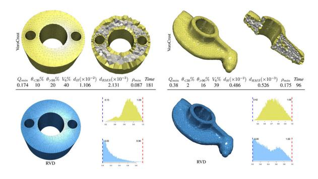
These images show 3D models created using VoroCrust, the first software that generates Voronoi-cell meshes without needing to be fixed manually. Researchers led by Sandia National Laboratories created the software. Credit: Sandia National Laboratories
