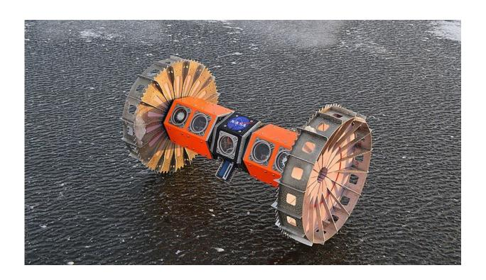
BRUIE (Buoyant Rover for Under-Ice Exploration) is an underwater rover prototype by NASA's Jet Propulsion Laboratory. The rover began testing in the Arctic in 2015 and it is meant to eventually explore the interior ocean of water worlds in the Solar System. BRUIE is buoyant and uses its two wheels to roll along beneath the ice and look for life. CC0 Public Domain
