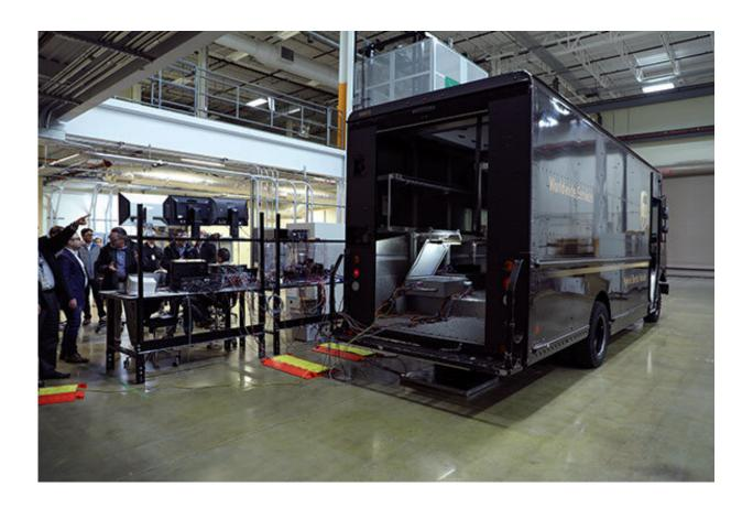
Oak Ridge National Laboratory researchers demonstrated on Feb. 27 a 20-kilowatt, bi-directional wireless charging system on a medium-class hybrid electric delivery truck. Credit: Brittany Cramer/Oak Ridge National Laboratory, U.S. Dept. of Energy
