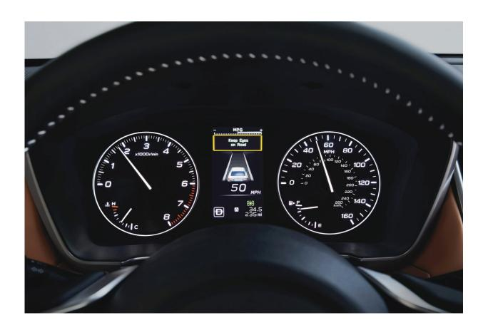
This photo provided by Subaru shows the driver attention monitor in the 2020 Subaru Legacy. It displays this warning when it detects the driver is not paying attention to the road. (Courtesy of Subaru of America via AP)
