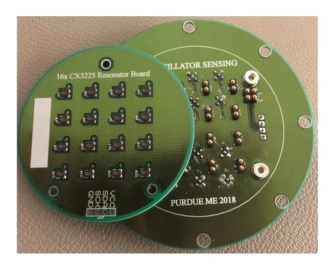
Purdue University researchers developed a sensor to help control and cut down on energy consumption through heating and ventilation systems, particularly those used in large office and hospitality industry buildings. Credit: Purdue University/Jeff Rhoads
