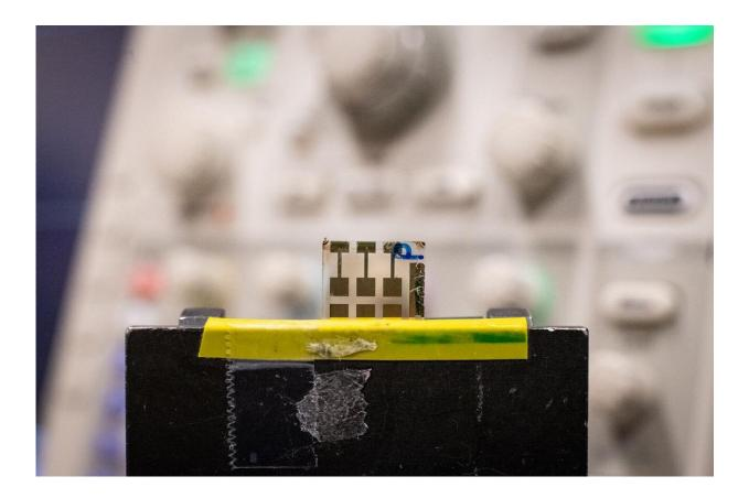
The tiny unit that can both receive and transmit optical signals. Credit: Magnus Johansson
