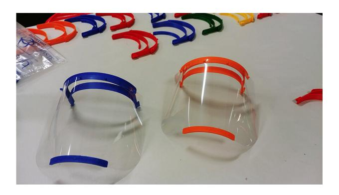
Engineers from the University of Sheffield are using 3-D printing techniques to make face shields for frontline NHS workers. Credit: University of Sheffield
