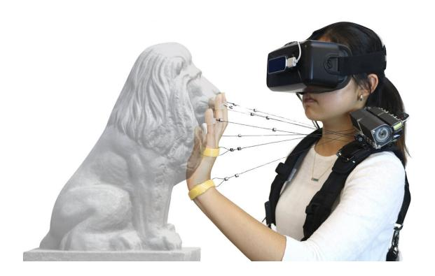
A new device developed at Carnegie Mellon University uses multiple strings attached to the hand and fingers to simulate the feel of obstacles and heavy objects in virtual reality environments. Credit: Carnegie Mellon University
