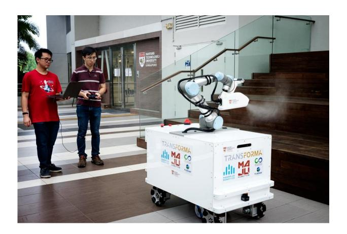
NTU's XDBOT can disinfect large surfaces quickly and can operate 4 hours continuously with its large disinfection tank and rechargeable batteries. Credit: NTU Singapore
