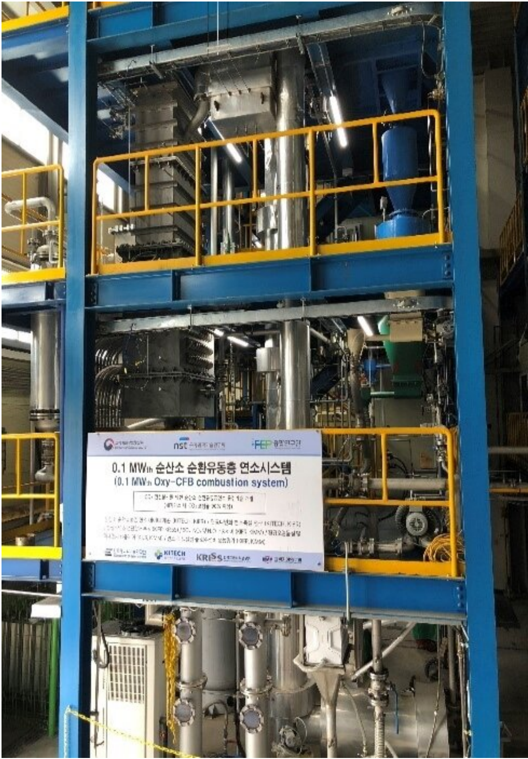
Oxy-Circulating Fluidized Bed Combustion system is an eco-friendly advanced power generation technology to meet the challenge of climate change. It can separate CO 2 during the combustion process, use various types of fuels and significantly reduce exhaust gas and air pollutants emission. Credit: Korea
