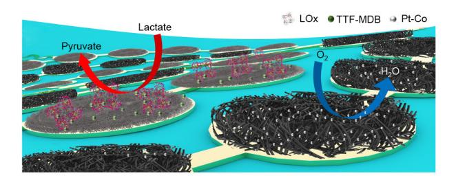
Schematic depicting a close-up of a soft biofuel cell array consisting of anodes and cathodes. Credit: Yu et al., Sci. Robot. 5, eaaz7946 (2020)
