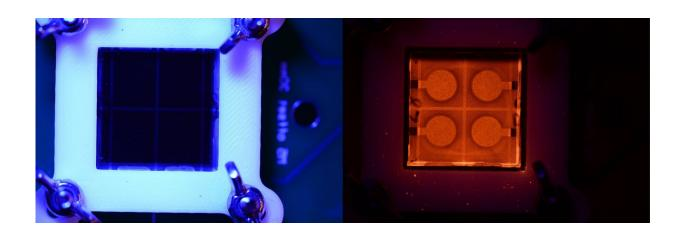
Perovskite solar cells bathed in blue light, and responding in infrared. Credit: Exciton Science
