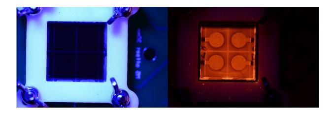
Perovskite solar cells bathed in blue light, and responding in infrared. Credit: Exciton Science
