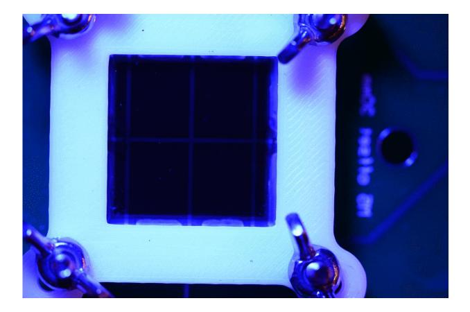
Perovskite solar cells in alternating blue and infrared. Credit: Exciton Science/Science in Public
