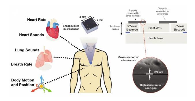
On the right, the minuscule gap that allows the Lilliputian chip to collect high-resolution signals from the broad array of sound and motion sources on the left. Credit: Georgia Tech / Ayazi lab
