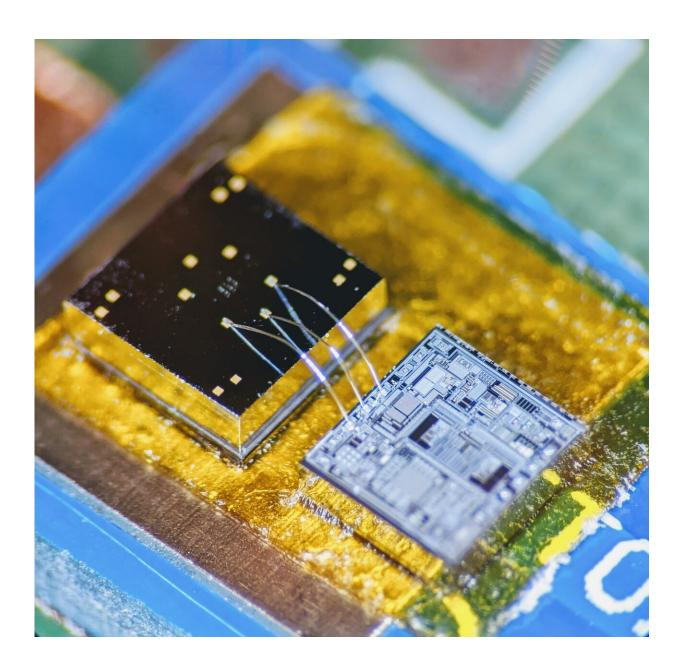
The sensor is a physical chip remarkably attuned to inertia. Next to it, an
