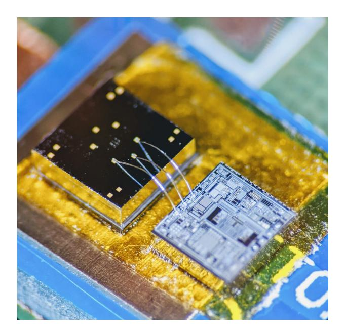
The sensor is a physical chip remarkably attuned to inertia. Next to it, an
