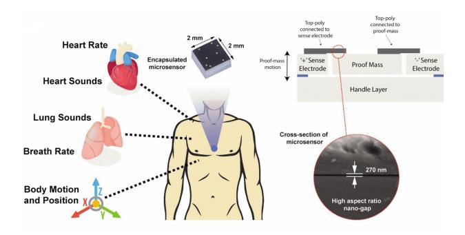
On the right, the minuscule gap that allows the Lilliputian chip to collect highresolution signals from the broad array of sound and motion sources on the left. Credit: Georgia Tech / Ayazi lab
