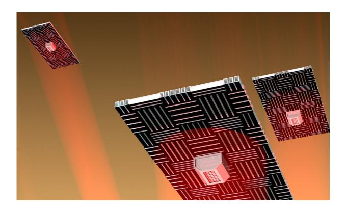
Despite weighing about a third of a milligram, Penn Engineers are now testing their "nanocardboard" flyers ability to lift payloads. In this artist's conception, fleets of flyers could be launched from ground-based rovers and steered with lasers to collect samples. Planets and moons with thin atmospheres and low gravities would enhance these flyers' ability to levitate by shooting air through their corrugated channels. Credit: Bargatin Group, Penn Engineering
