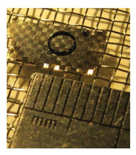
Nanocardboard's corrugated channels provide stiffness, but are also responsible for its ability to levitate, as creating a temperature differential generates an air current that flows through its hollow structure. A recent study allowed Penn Engineers to measure the flyers' ability to lift mock payloads (silicone rings, attached to the top of the plates) thanks to a new low-pressure test chamber with integrated cameras and light sources. Credit: Bargatin Group, Penn Engineering
