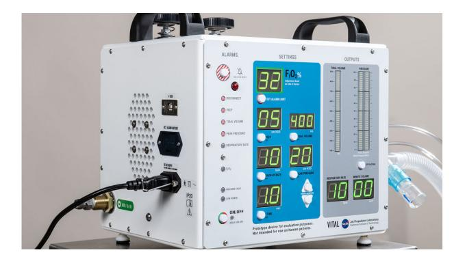
This image shows the ventilator prototype for coronavirus patients designed and built by NASA's Jet Propulsion Laboratory in Southern California. Credit: NASA/JPL-Caltech
