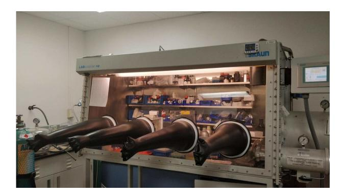
A glovebox used for testing the batteries. Credit: The University of Texas at Austin
