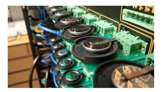
This battery cycler in Arumugam's Manthiram's lab can test multiple coin cells at the same time. Credit: University of Texas at Austin
