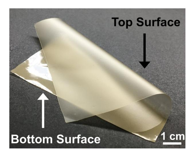
The top surface of the pollen paper, which appears frosted to the naked eye, has a relatively rougher surface as compared to the bottom surface, which takes on a mirror-like surface finish. This structural difference in pollen particle layers means that in the presence of water vapour the paper starts to bend, and under dry conditions, it unbends. Repeated cycles of humid and dry conditions cause
