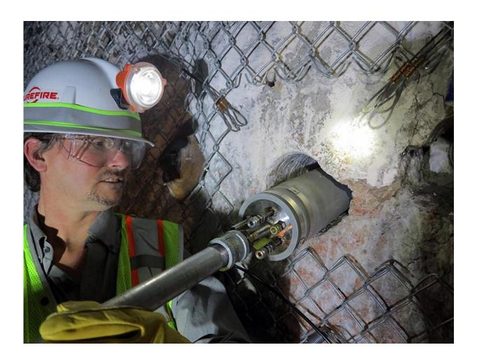
Phil Stauffer testing the inflatable packer fit into the BATS testing borehole. This is a mock-up waste canister filled with cerabeads (fake nuclear waste, with properties like glass) and heater strips to mimic 1000W of heating. The project hopes to find solutions for nuclear waste storage in salt deposits deep in the earth. Credit: Doug Weaver
