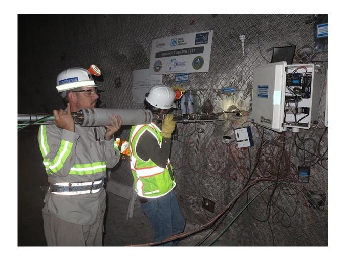
Installation of the infrared heater being tested at a one of the BATS research sites. Credit: Doug Weaver
