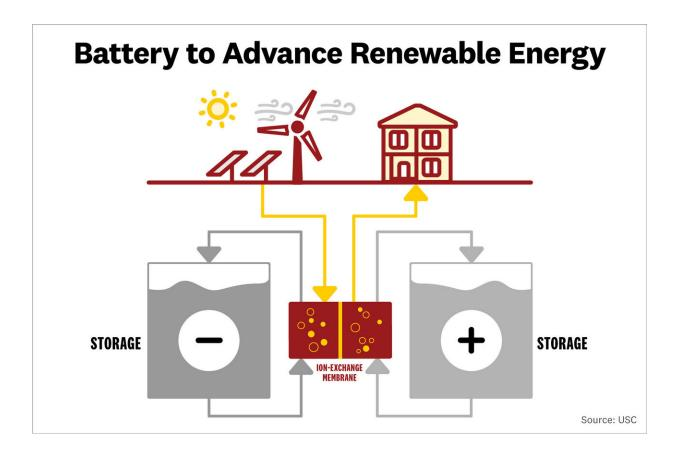
How the redox flow battery works. Credit: USC
