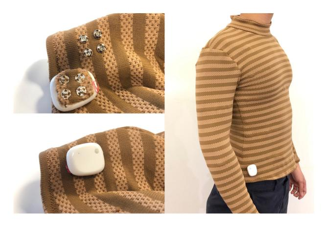
The conformable garment ensures robust sensor-to-skin contact while keeping the clothing comfortable. A detachable wireless module allows you to easily charge and wash the garment. Credit: MIT Media Lab
