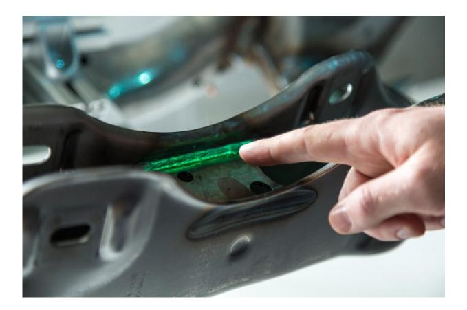
The position of weld seam defects identified by the user can be determined by a combination of finger tracking and 3D seam tracking, and precisely documented. Credit: Fraunhofer HHI
