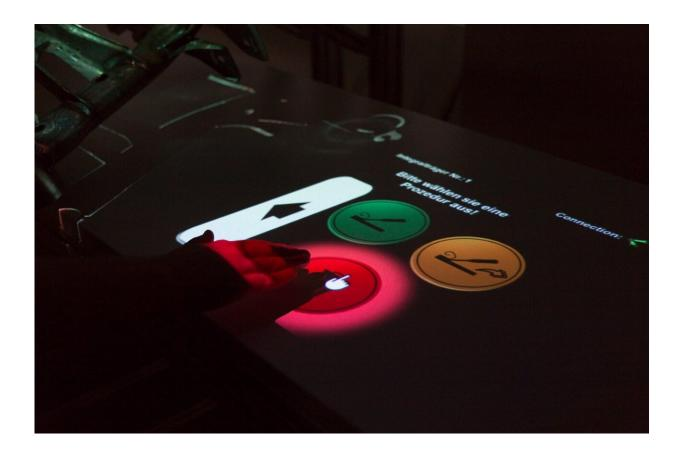
An augmented hand gesture-based user interface is projected onto the component and workbench, where it serves to control the robot and the inspection procedure. Credit: Fraunhofer HHI
