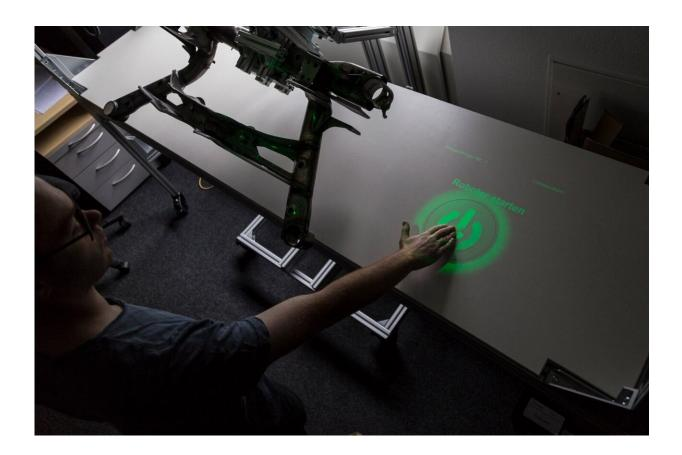
The robot presents the workpiece in an ergonomic position to enable easy inspection. Credit: Fraunhofer HHI
