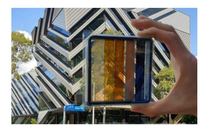
A semi-transparent perovskite solar cell with contrasting levels of light transparency. Credit: Dr Jae Choul Yu
