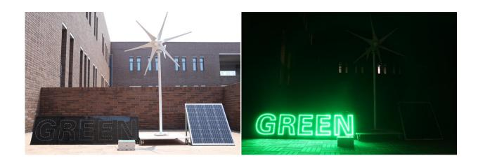
Demonstration of a renewable energy storage system. Photos of the researchers' demonstration of a renewable energy storage system based on a DZMB pack (in the middle of the photo) integrated with solar photovoltaic (PV) modules and a wind-driven generator through a controller. The controller was also connected to a light-emitting diode (LED) panel, serving as the electrical load. Credit: Zhong et al.
