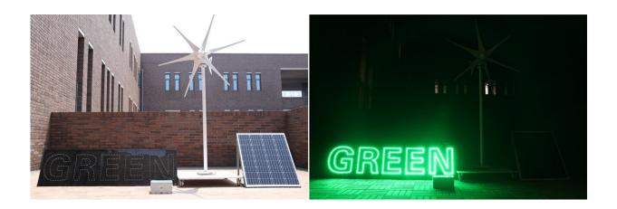
Demonstration of a renewable energy storage system. Photos of the researchers' demonstration of a renewable energy storage system based on a DZMB pack (in the middle of the photo) integrated with solar photovoltaic (PV) modules and a wind-driven generator through a controller. The controller was also connected to a light-emitting diode (LED) panel, serving as the electrical load. Credit: Zhong et al.
