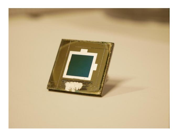
The CIGS-Pero tandem cell was realised in a typical lab size of 1 square centimeter. Credit: HZB
