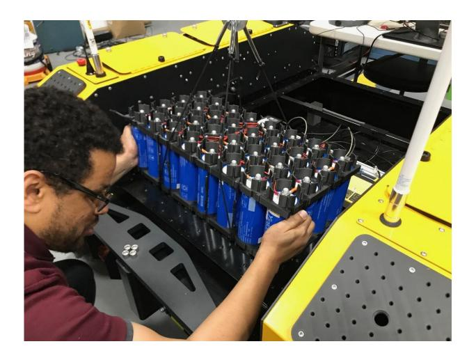
Army Electrical Engineer Wosen Wolde installs the 2.5 kilowatt-hour lithium battery system designed by CCDC Army Research Laboraory. Here, Wolde lowers the battery into a test vehicle using an engine hoist. The battery fills up one-third of the vehicle's internal volume. Credit: CCDC Army Research Laboratory
