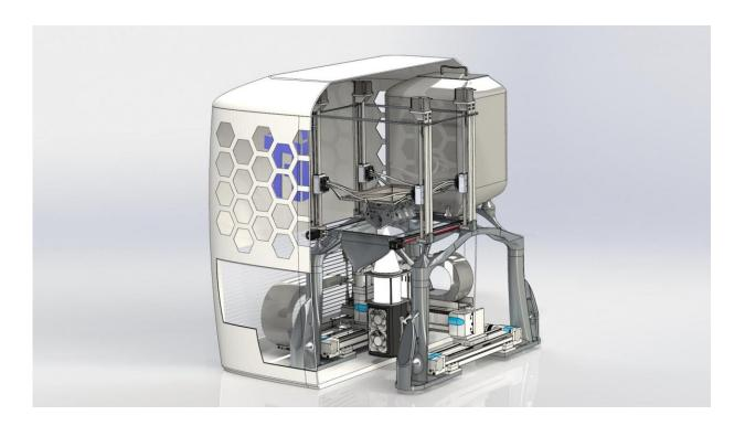
The 3D printer developed at TU Graz melts metal powder using highperformance LED light sources and then processes it into components in additive manufacturing. Credit: TU Graz
