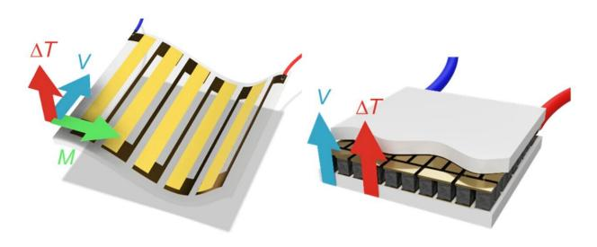
Thermoelectric devices based on the anomalous Nernst effect (left) and the Seebeck effect (right). (V) represents the direction of current, (T) the temperature gradient and (M) the magnetic field. Credit: © 2020 Sakai et al
