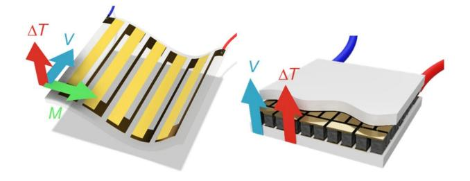
Thermoelectric devices based on the anomalous Nernst effect (left) and the Seebeck effect (right). (V) represents the direction of current, (T) the temperature gradient and (M) the magnetic field. Credit: © 2020 Sakai et al
