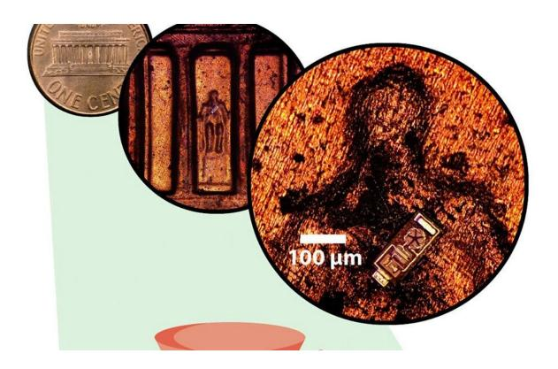
This image shows a voltage-sensing OWIC as it fits inside the Lincoln Memorial on the back of a penny, and a schematic of an OWIC's components. Credit: Alejandro Cortese
