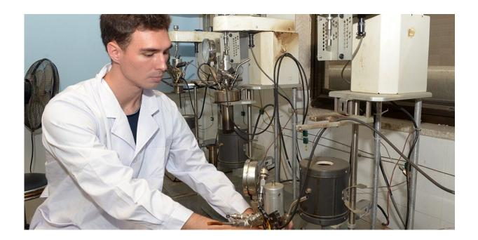
Jamison Watson, doctoral student in agricultural and biological engineering, prepares a hydrothermal liquefaction batch reactor for the conversion of algae into biocrude oil and wastewater. Credit: University of Illinois at Urbana-Champaign
