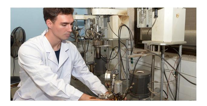
Jamison Watson, doctoral student in agricultural and biological engineering, prepares a hydrothermal liquefaction batch reactor for the conversion of algae into biocrude oil and wastewater. Credit: University of Illinois at Urbana-Champaign
