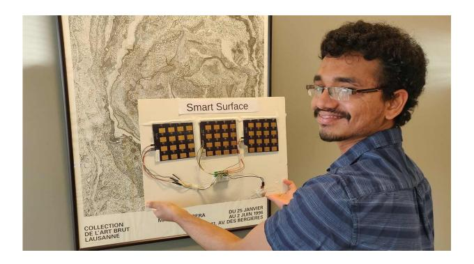
Manideep Dunna, a UC San Diego electrical and computer engineering Ph.D. student, holds a prototype "smart surface" that can be stuck on the wall to improve WiFi connectivity in the home and office. Credit: University of California - San Diego
