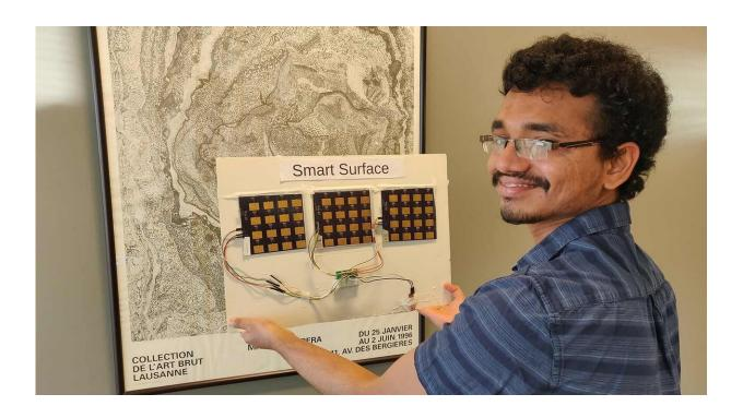
Manideep Dunna, a UC San Diego electrical and computer engineering Ph.D. student, holds a prototype "smart surface" that can be stuck on the wall to improve WiFi connectivity in the home and office. Credit: University of California - San Diego
