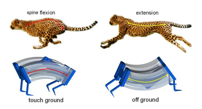
Inspired by the biomechanics of cheetahs, researchers have developed a new type of soft robot that is capable of moving more quickly on solid surfaces or in the water than previous generations of soft robots. Credit: Jie Yin, NC State University
