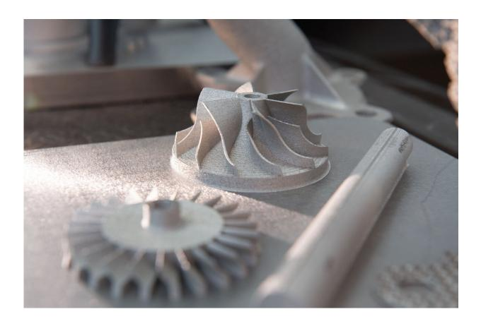
Army researchers study the performance of 3-D-printed metal parts and how they degrade as part of ongoing research in vehicle technology. The CCDC Army Research Laboratory at Aberdeen Proving Ground, Maryland, prints metal parts from powder. Credit: Dave McNally
