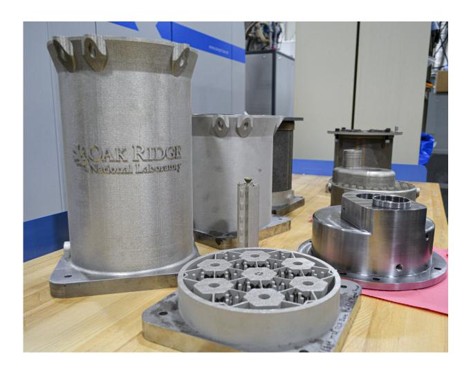
ORNL scientists have selected and optimized a design for printing over a three month period, demonstrating the ability to rapidly produce a prototype reactor core. Credit: Brittany Cramer/Oak Ridge National Laboratory, U.S. Dept. of Energy
