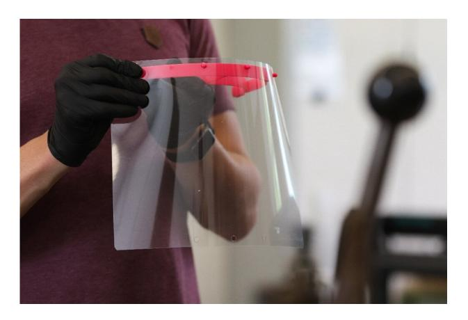
3D printers fabricate the red piece that holds a sheet of transparent plastic
