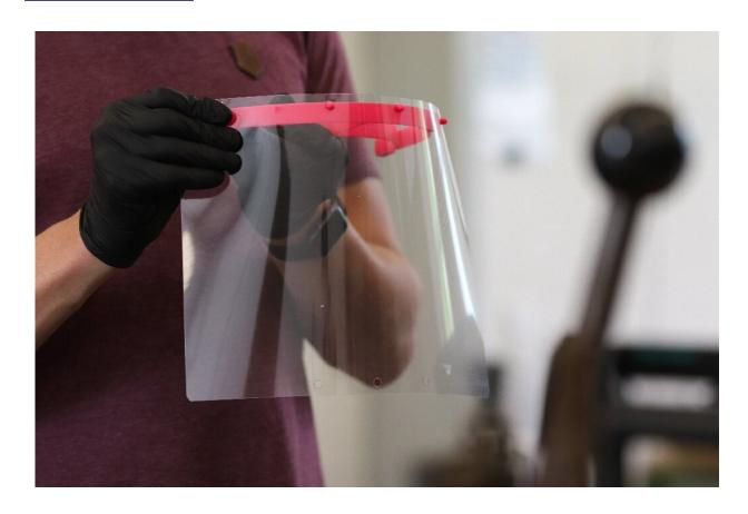
3D printers fabricate the red piece that holds a sheet of transparent plastic
