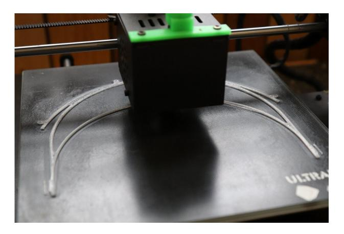
3D printers fabricate by deposing layer upon layer of material, and can be quickly reprogrammed to produce different pieces
