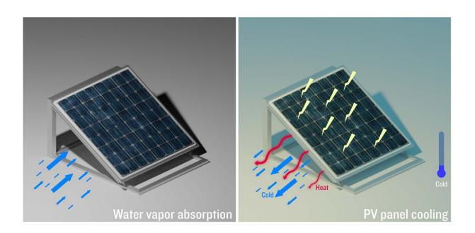
When the gel is fully filled with water, it can free enough water to reduce panel temperatures by 10 degrees Celsius. Credit: © 2020 KAUST; Youssef A. Khalil
