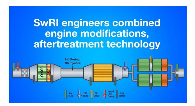
Southwest Research Institute engineers have developed the next generation of clean diesel engine technology to reduce hazardous nitrogen oxides  $(NO_x)$  and carbon dioxide emissions while minimizing fuel consumption. Working with regulatory agencies, vehicle manufacturers and suppliers, SwRI combined engine modifications with integrated aftertreatment technology and control strategies to reach near-
