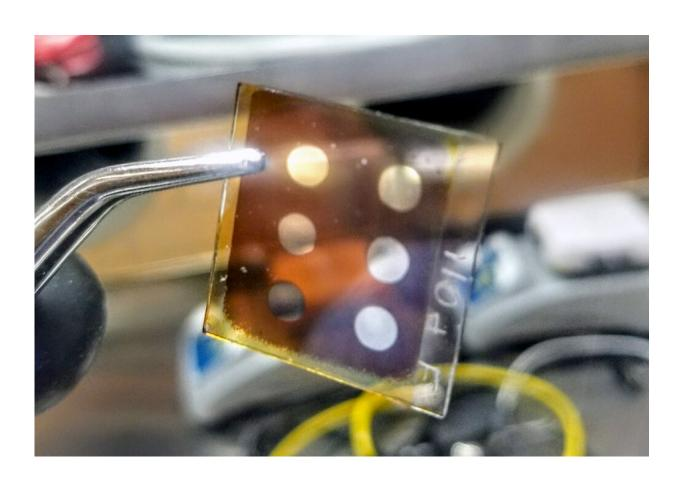
Iowa State engineers fabricated this proof-of-concept perovskite solar cell in their research lab. Credit: Harshavardhan Gaonkar
