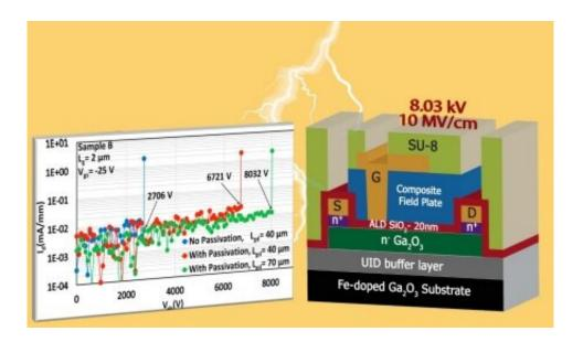
The graph image on the left shows the breakdown voltage of three different versions of the gallium oxide transistor. The illustration on the right shows the configuration and materials that make up the transistor that achieved a breakdown voltage of more than 8,000 volts. Credit: University at Buffalo
