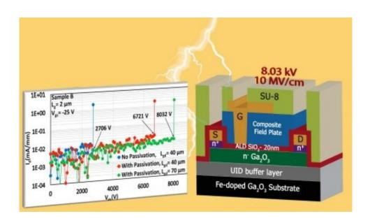
The graph image on the left shows the breakdown voltage of three different versions of the gallium oxide transistor. The illustration on the right shows the configuration and materials that make up the transistor that achieved a breakdown voltage of more than 8,000 volts. Credit: University at Buffalo
