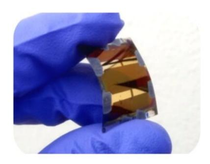
A curved perovskite photovoltaic cell on ultra-thin flexible glass. Credit: Cell Press
