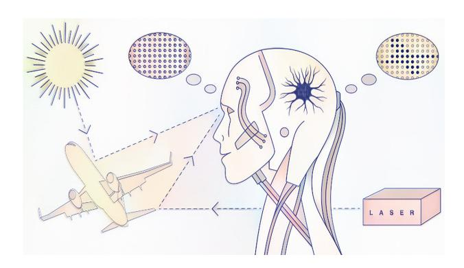
A detector (the eye) measures identical photons from natural sunlight and laser light. The fast identification of light sources is performed by an artificial neuron that is trained to efficiently extract patterns in the quantum fluctuations of photons. Credit: Elsa Hahne
