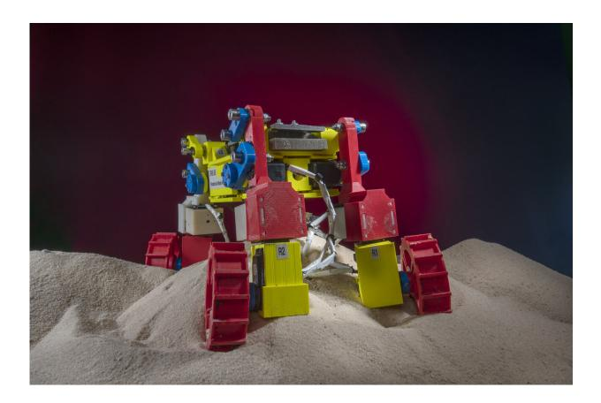
Built with multifunctional appendages able to spin wheels that can also be "wiggled" and lifted, the Mini Rover was modeled on a novel NASA rover design and used in the laboratory to develop and test complex locomotion techniques robust enough to help it climb hills composed of granular material, here ordinary beach sand. Credit: Christopher Moore, Georgia Tech
