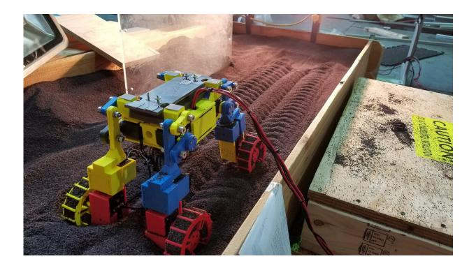
The Mini Rover moves through a bed of poppy seeds designed to model movement through granular surfaces. The robot was used to test complex locomotion techniques robust enough to help it climb planetary or lunar hills covered with such granular material. Credit: Goldman lab, Georgia Tech
