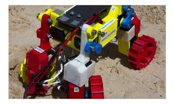
Built with multifunctional appendages able to spin wheels that can also be "wiggled" and lifted, the Mini Rover was modeled on a novel NASA rover design and used in the laboratory to develop and test complex locomotion techniques robust enough to help it climb hills composed of granular material, here ordinary beach sand. Credit: Christopher Moore, Georgia Tech
