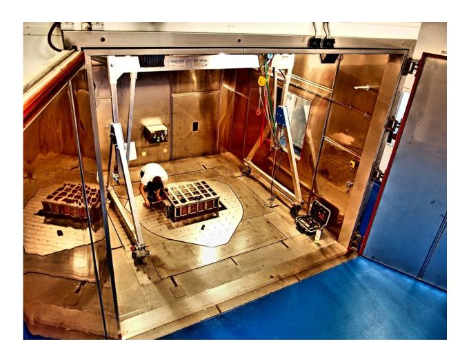
Battery test bench at Fraunhofer LBF. Credit: Fraunhofer LBF
