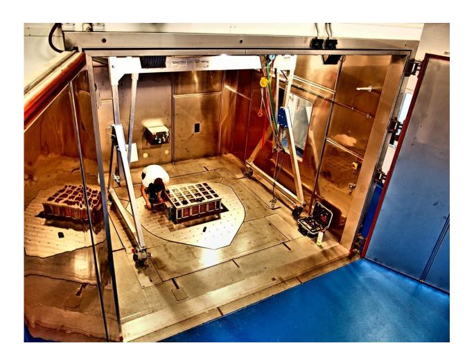
Battery test bench at Fraunhofer LBF. Credit: Fraunhofer LBF
