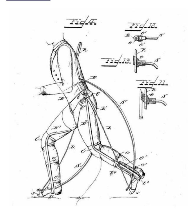
In 1890, Nicolas Yagn invented a spring-leg that supported the weight of a person's body. Credit: USPTO
