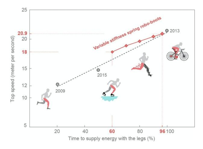
Top speed of human-powered locomotion. Credit: Adapted from A. Sutrisno, D. J. Braun, How to run 50% faster without external energy, vol. 6, no. 13, eaay1950, 2020., <u>CC BY-ND</u>
