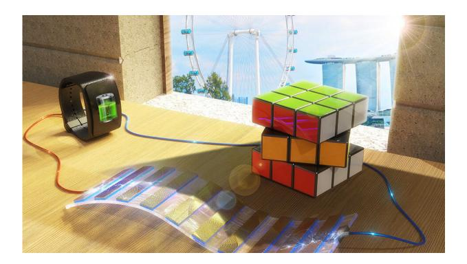
The novel shadow-effect energy generator developed by NUS researchers uses the contrast in illumination between the lit and shadowed areas to generate electricity. Credit: Royal Society of Chemistry
