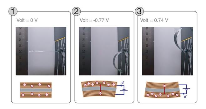
A new carbon fibre composite material which can be bent with electronic impulses was demonstrated in a recent proof-of-concept study. Credit: KTH The Royal Institute of Technology
