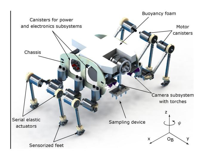
Schematic of SILVER2's design. Credit: Picardi et al., *Sci. Robot.* 5, eaaz1012 (2020)
